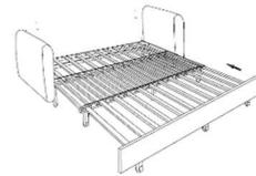
There are 2 holes at back corner of seat frame, attach backframe into the seat frame(No screws needed).
